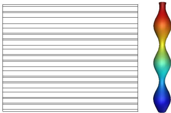
Figure 5: Periodic column of revolution with up-down reflection.
