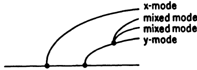
Figure 1.3. Schematic bifurcation diagram when symmetry-breaking terms are included.
